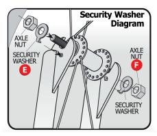
Removing the front wheel is quite straightforward, all you need do is untighten the wheels nuts it ill slack enough to release the safety locking washers to you to lift the wheel out of the drop-outs in the fork. You do not need to remove the nuts completely.
