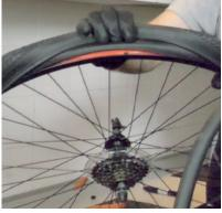
Pull the tyre back to reveal the hole in the rim for the valve
