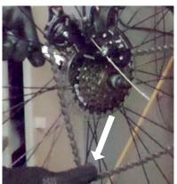
Firstly pull the lower loop of chain down underneath the cogs on the wheel.
