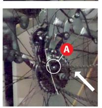
Bring your wheel up so that chain sits on top of the smallest cog of the wheel next to the upper jockey wheel A which is closest to the body of the mechanism
