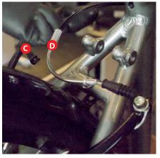
Slide back the dust cover (A) which reveals the brake cabel. Using your hand pull the brake levers (B) together until you can pull the cable bridge (C) down releasing the cable guide (also called a noodle) (D) taking care not to bend it or the cable will not slide through it.
