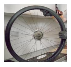
Fitting the tyre the wrong way round will effect the wet grip, breaking distance and cornering grip of the tyre.
