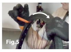
**Fig.5** Whilst holding the tyre firmly in place with your left hand place the tyre lever as shown, only lifting approx. 90 degrees to the rim and slowly working toward the valve as the tyre pops inside the rim. If it feels difficult, reverse, by holding the tyre with your right hand and work toward the valve from the other direction until the whole tyre pops in place inside the rim.
