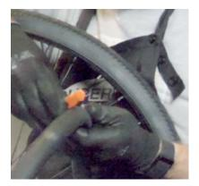
Reduce some of the air from the innertube using the tyre lever.
