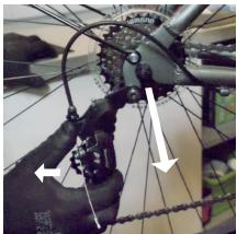
Push the mechanism back and the wheel can be easily removed.
