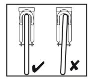
Centralizing the wheel correctly before tightening the wheel nuts
