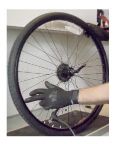
What you need to do is check that the beading around the tyre looks like it is sitting equally, and you need to check both sides of the tyre.
