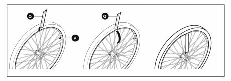
**NOTE:** To remove the innertube you will need a set of tyre levers
